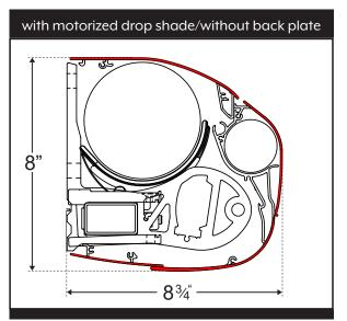
\*Can be roof mounted with 12" roof mounting brackets.
